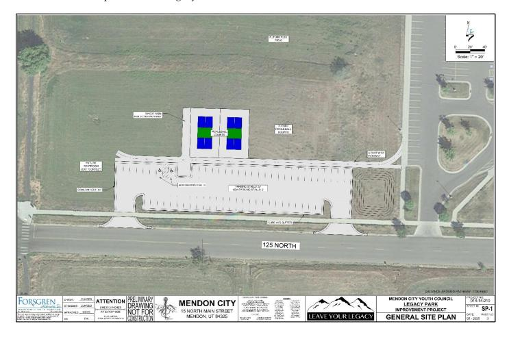
They will front the parking lot with a sidewalk that extends down the side of the pickleball courts. They have reduced the parking stalls from 63 to 57. The map shows a paved parking lot, curb and gutter,
